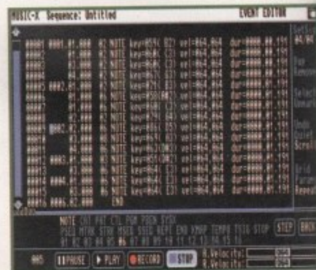
Each separate Midi event can be seen here, in Music-X, giving information about the time, duration and pitch of the note etc
